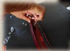
You will need to enlarge the hole in the center for the electrical connector to the light. The new spoiler fits differently. You need to remove quite a bit of the plastic.
