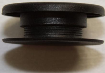
If this happens to you, the quick fix is to simply move the left retainer to the right side, but it does require you have a screwdriver or other prying instrument to separate the retainers. The picture at left shows how they go together. There are actually three of these retainers on the trunk partition (the third is on the bottom right by the passenger seat back—but that is very hard to get to).
