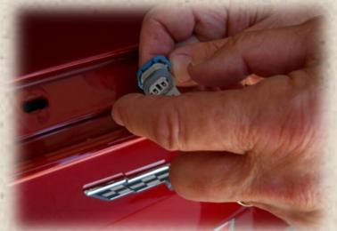
Remove the light from the old spoiler and install it in the new spoiler. Use the long bolts from the spoiler you removed, rather than the two small black screws that came with the spoiler. When installing these screws place 3 small washers under the screws. This will make the screws long enough to allow for the nuts to be installed. *Note - This is important or the screws will not protrude through the body far enough to install the nuts!*
