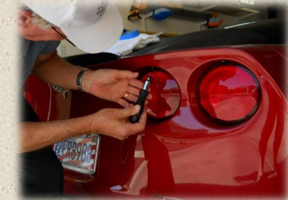
Take out all four tail lights. This makes it easier to reach the screws (Trox) that hold the current spoiler in and then installing the new bolts.
