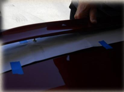
Before drilling - Perform an alignment test fit of the spoiler to see if the screw placement matches the drilling location marks on the template. Ours was off a bit so we had to make adjustments on the template.
