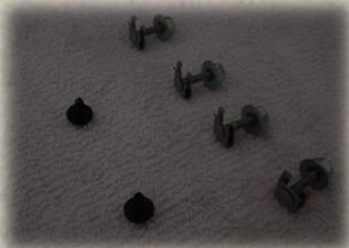
These are the four long bolts and two small black screws that came with the new spoiler. We did not use the two small ones.
